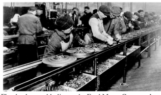
Flywheel assembly line at the Ford Motor Company's MI in 1913 [Politico].
